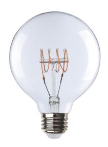
Truefila is an upgraded LED filament bulb. By using polyimide flexible material as a substrate, the flexible filament has higher flexibility and a larger luminous coverage area under 0.6mm substrate, making the bulb achieve free 360° luminescence.
