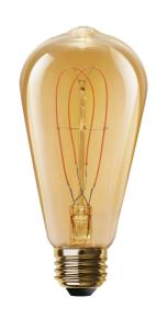
Truefila is an upgraded LED filament bulb. By using polyimide flexible material as a substrate, the flexible filament has higher flexibility and a larger luminous coverage area under 0.6mm substrate, making the bulb achieve free 360° luminescence.
