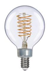
Truefila is an upgraded LED filament bulb. By using polyimide flexible material as a substrate, the flexible filament has higher flexibility and a larger luminous coverage area under 0.6mm substrate, making the bulb achieve free 360° luminescence.
