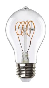
Truefila is an upgraded LED filament bulb. By using polyimide flexible material as a substrate, the flexible filament has higher flexibility and a larger luminous coverage area under 0.6mm substrate, making the bulb achieve free 360° luminescence.
